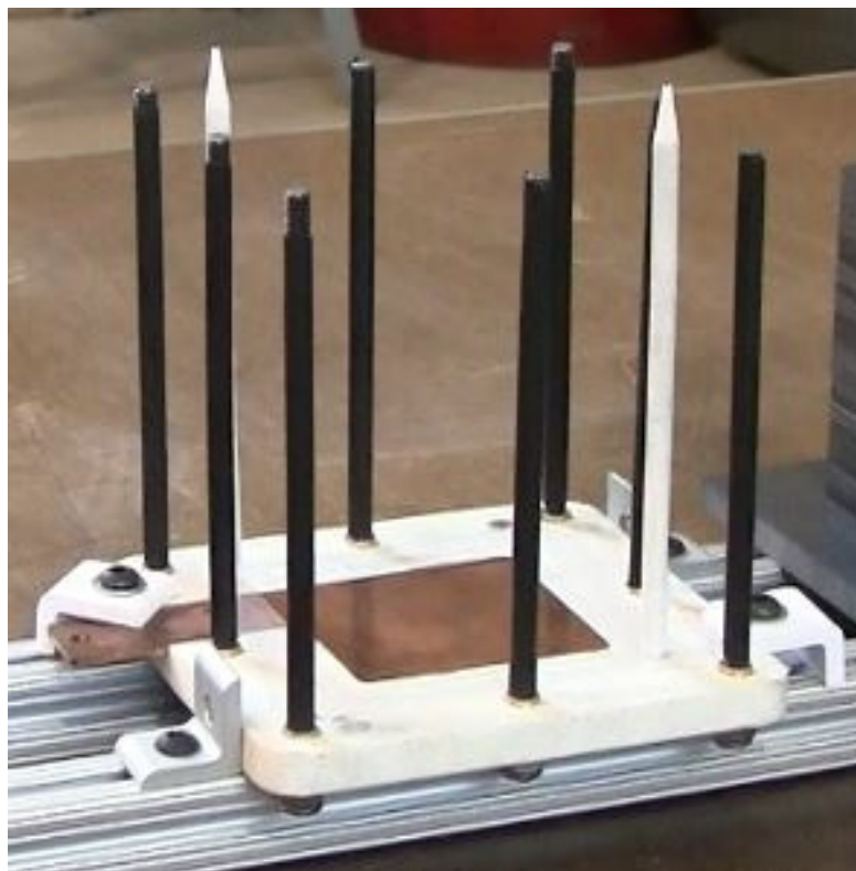
Figure 4. Endplate located and clamped in the assembly workcell. Two poly(tetra)fluoroethylene (PTFE) alignment pins (white) are permanently mounted on the endplate. The alignment pins feature a conical end which eases the engagement between the positioning holes on the end-effector and fuel cell components and the alignment pins during release operations. There are also eight tie-rods mounted on the endplate which used for compressing the stack. The figure also depicts two locators and two clamps used for positioning the endplate on the workbench.
